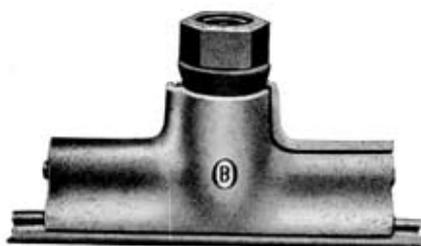
**T**WO interlocking jaws are hinged on a steel pin which passes through lower end of stud bolt. Special nut is cone-shaped on one end to correspond to a recess on top of Clamp, and hexagonal on other end so that the Type D Wrench may be used on it.
