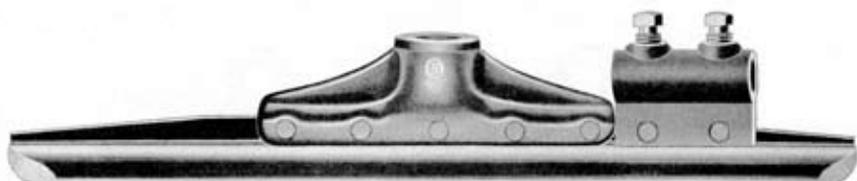
**S**IMILAR to regular Extruded Ear described on preceding pages with addition of a horizontal bronze feeder lug drilled to accommodate No. 2-0 to 4-0 B. & S. solid or stranded wire.
