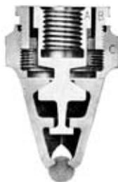
**A**LWAYS fits tightly against hanger when aligned with wire. To install, screw onto hanger stud until boss (A) is in contact with trolley hanger. Then back off to align with wire, insert wire and tighten nut (C). Sleeve (B) then fits tightly against bearing surface of hanger.
