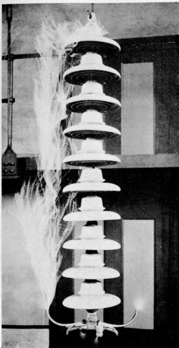
**O**-B Suspension Insulators—10 Units No. 25622 with Suspension Clamp No. 11549—flashing at nearly 500,000 volts. Were it desirable, this flash-over point could be increased materially by increasing the spacing between the individual units.
