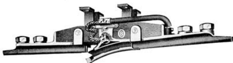
**I**NTENDED for use in mines where it is desired to keep the trolley on any section alive only when a locomotive is operating in that section. The function of the device is to automatically close the circuit as locomotive enters upon the section and to open it as locomotive passes out.
