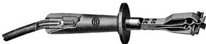
**D**ESIGNED for connecting welding or cutting machine to mine trolley. The connector has a steel spring which holds the copper lips tight against the wire.
