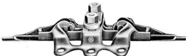
**W**IRE is gripped firmly by clamp casting held in place by two  $\frac{3}{8}$  x  $1\frac{1}{2}$ -inch standard carriage bolts equipped with lock washers. Clamp is serrated to give great holding power.
