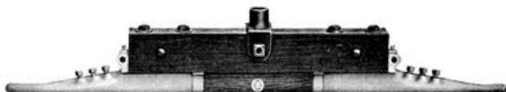
**B**ODY portion is a heavy block of thoroughly seasoned hickory impregnated and varnished to which bronze end castings are securely bolted. The outer ends of these castings are grooved at bottom to receive trolley wire, which is fastened in place by means of set screws.
