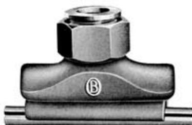
**C**ONSISTS of two substantial jaws with their upper portions interlocking and held together by a high strength steel rivet, upon which the jaws have a hinge action, clamping upon the wire by means of a yoke casting which is forced down upon them by a hex nut threaded on outside of boss.
