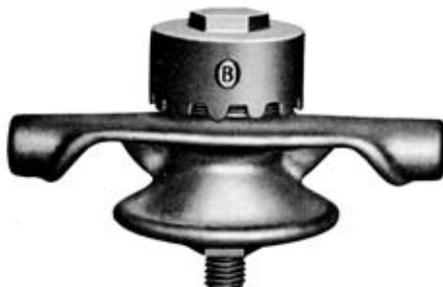
**P**REFERRED to D-1 Hanger where conditions are particularly severe. Body portion is heavier than D-1 and broader skirt affords increased protection to lower end of insulated bolt. Arms are reinforced by webs.
