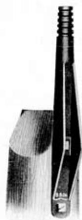
**C**ONSISTS of two malleable iron castings fastened together by a threaded stud screwing into both. Thimbles may be cemented into insulators at factory, castings mounted on poles and insulators installed at any time.
