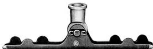
**O**FFERS a flexible support for wire on straight line work. To install, remove swiveled boss, place trolley wire in groove and bend lips over it, finally replacing boss and attaching Ear to hanger. Can be used to advantage where several styles of wire are found on the same line.
