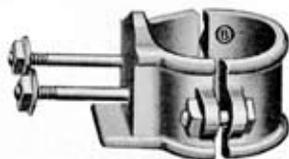
USED for attaching standard size wood cross arms to iron poles. The cross arms are secured to the supports by the two  $\frac{1}{2}$ -inch bolts shown, which pass through them and clamp them in place by means of a nut and washer on their outer ends. These supports are made of malleable iron, japanned.
