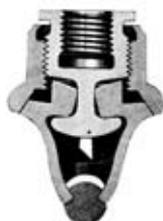
IS screwed on to the hanger and backed off until clamp aligns with the wire. The only necessary operations in installing this clamp are; insert the wire in the jaws of the clamp, then tighten the nut making a positive grip.
